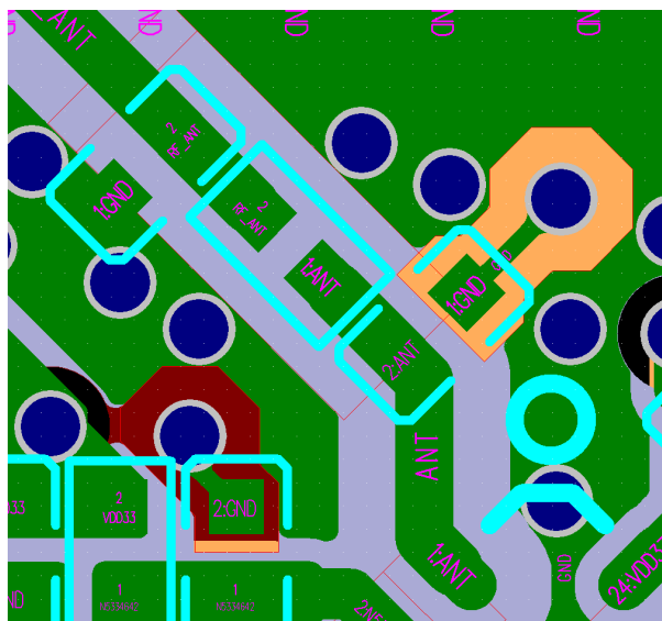
Fig. 14: ESP32-C2 Stub in a Four-layer PCB Design
